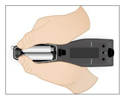
The battery compartment holds a battery block with 4x LR6 (AA) alkaline Mignon batteries (Industrial by Duracell recommended). As a general rule, all four batteries should be replaced at the same time. Ensure the polarity of the batteries is correct. The battery block is then reinserted into the case. The battery block connections (arrow) must face towards the device and be on top as shown in the following image. The battery compartment cover can now be closed again.
