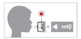
The red LED illuminates to indicate that the internal memory is full. The full state is also indicated with a beep.
