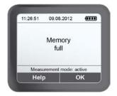
After the 9,999th measurement, the message "Memory full" appears on the display. If any further measurements are taken, a query appears asking whether old data should be overwritten. This has to be confirmed once by pressing >YES< or >NO< and does not appear again until the device is restarted.
