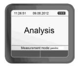
The yellow LED is flashing during the evaluation of the breath sample. Depending on the alcohol concentration this can take several seconds.
