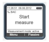
Select the >passive measurement mode< by pressing the >Passive< key or via the menu.
