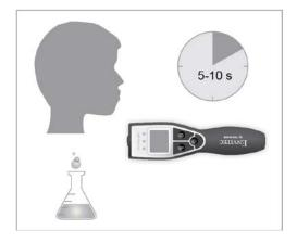
Place the device which is ready to take measurements (without mouthpiece) close to the point to be measured (e.g. in front of the patient's mouth and nose) for about 5–10 seconds (s).
