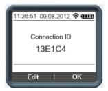
Having selected the option >Wireless<, an appropriate wireless printer can be used. Prior to the initial wireless operation, the printer and the AlcoQuant 6020 plus need to be paired with each other by using the Connection ID of the printer. The single digits of the printer Connection ID have to be set with the key >Edit<. Finally confirm the Connection ID with >OK<. A printer test can then be performed with >Print<.
